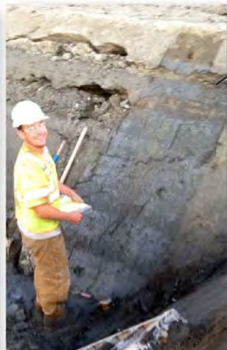
View of Alternating Sand, Silt, and Clay Layers Exposed East of Skeleton to the Southwest (left) and West (right)
